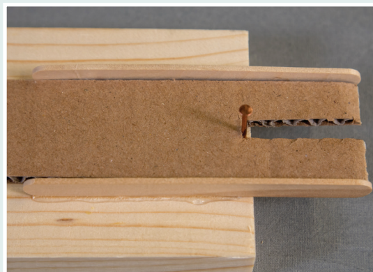
Figure 2: Popsicle sticks guide the cardboard, do not glue cardboard
